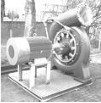
Francis Turbine and generator
